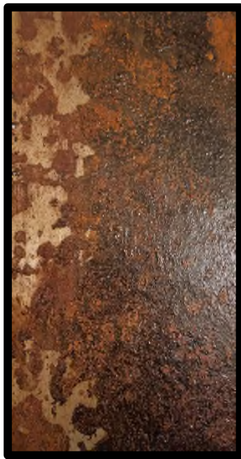
Blank Control Mineral Oil Brush Applied to a Sanded Q-Panel. 48 Hours Humidity, Horizontal Orientation.
